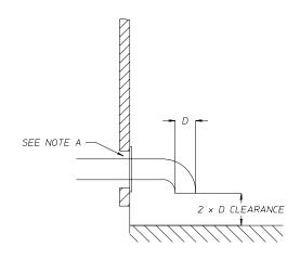
NOTE "A": OPENING MUST BE TWO (2) INCHES (5.08 CM) LARGER THAN DUCT (ALL THE WAY AROUND). THE DUCT MUST BE CENTERED WITHIN THIS OPENING.
